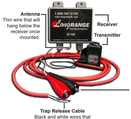
The LT-100 includes 1 receiver with a 1 button transmitter. The LT-200 includes 2 receivers with a 3 button transmitter. The 2 receivers included with the LT-200 will be labeled with Trap 1 and Trap 2. The receivers include 2 mounting holes and it is recommended that the receivers are mounted on a non-metal post, 2-3 feet high with the antenna hanging below the receiver.
